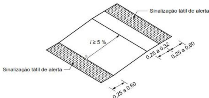
Figura 14 – Rampas fixas com  $i \geq 5\%$
